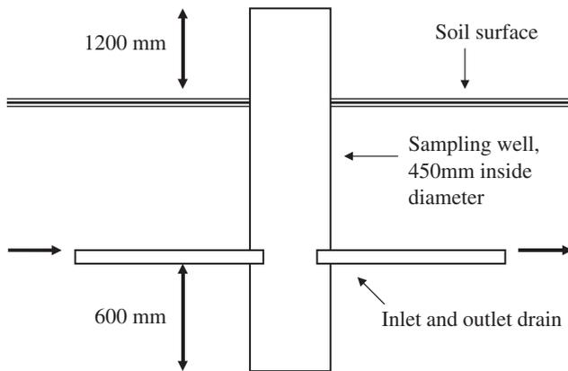
Fig. 2. Profile of the sampling well
